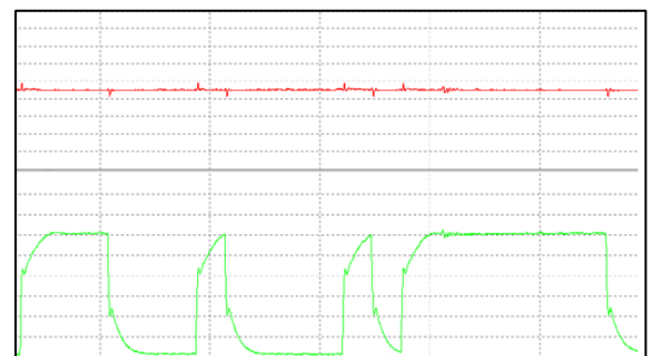
Figure 10: short-circuited A and B-line
